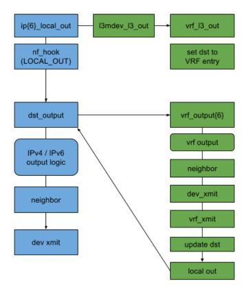
Figure 5. Transmit path for VRF.
