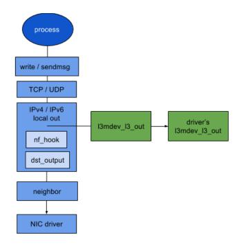
Figure 4. I3mdev transmit hook.
